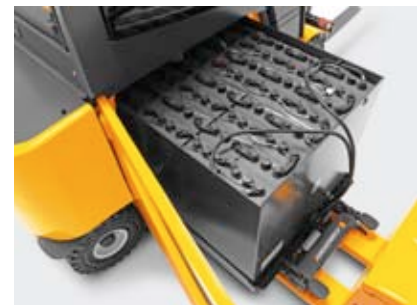
Battery removal with SnapFit
